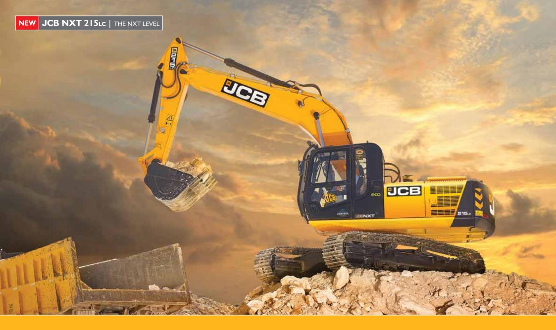
Gross engine power : 104 KW (140 hp), Bucket capacity : 0.8 cu.m - 1.02 cu.m Operating weight : 21,500 kg
